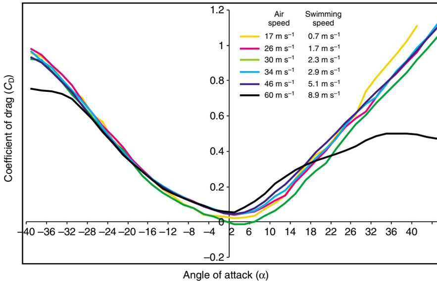
Fig. 5. Averaged drag data for the minke whale flipper model. Averaged wind tunnel measurements of the drag coefficient,  $C_D$ , shown as a function of the angle of attack,  $\alpha$ , on the x-axis at 17 m s<sup>-1</sup> (yellow), 26 m s<sup>-1</sup> (pink), 30 m s<sup>-1</sup> (green), 34 m s<sup>-1</sup> (light blue), 46 m s<sup>-1</sup> (indigo) and 60 m s<sup>-1</sup> (black).
