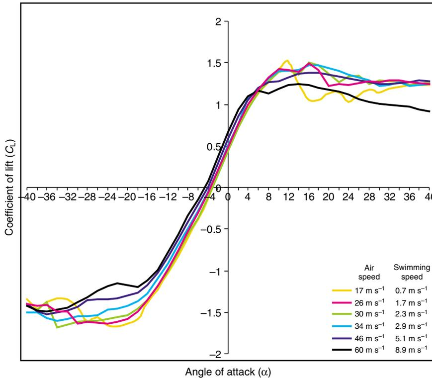
Fig. 4. Averaged lift data for the minke whale flipper model. Averaged wind tunnel measurements of the lift coefficient,  $C_L$ , shown as a function of the angle of attack,  $\alpha$ , on the x-axis at 17 m s<sup>-1</sup> (yellow), 26 m s<sup>-1</sup> (pink), 30 m s<sup>-1</sup> (green), 34 m s<sup>-1</sup> (light blue), 46 m s<sup>-1</sup> (indigo) and 60 m s<sup>-1</sup> (black).
